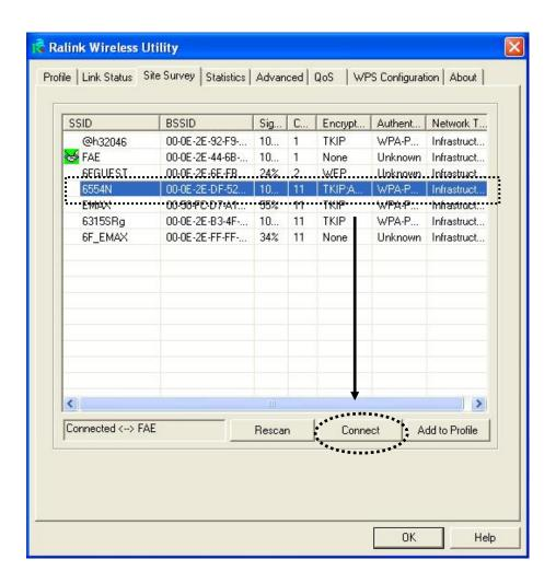
If the access point you selected does not enable encryption (The content of 'Encryption' field of the access point you selected is 'None', you'll be connected to this wireless access point within one minute. Please jump to step 6.
