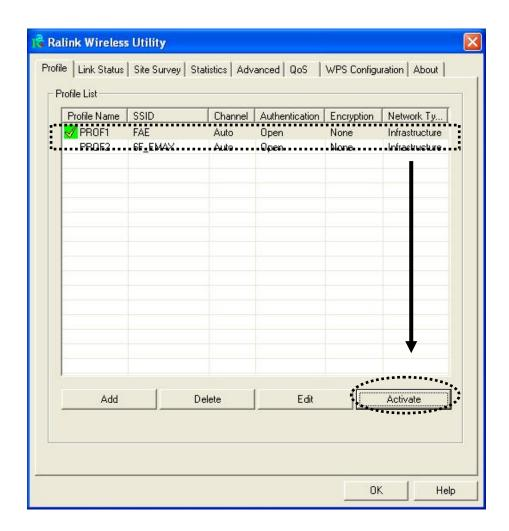
Select the profile you wish to use, and click 'Activate' to use the profile you selected. You can only activate a profile a time, and the profile which is activated currently will have a green check ( ) before its name. If the wireless access point is not reachable, a red check ( ) will be displayed before its name.
