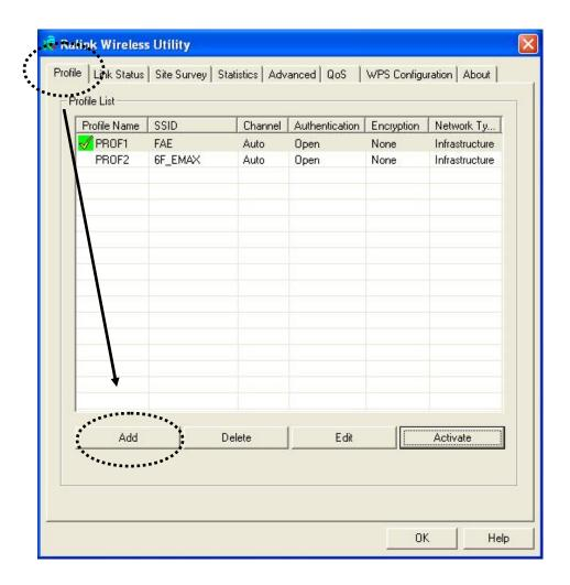
Or, you can add a connected wireless access point or wireless device to a profile by clicking 'Site Survey' tab, then click 'Add to Profile' button:
