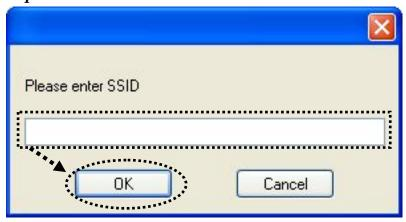
5. If the wireless access point uses encryption, you have to input WEP passphrase or WPA preshared key. Please ask the owner of the wireless access point you want to connect, and input the correct passphrase / preshared key here, then click 'OK'. If the value you inputted here is wrong, you will not be able to connect to this wireless access point.
